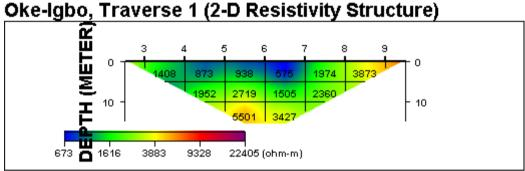
Fig. 3: Inverse resistivity model along Traverse 1 across the landslide
