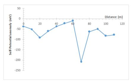
Fig. 10: SP anomaly plot for Traverse 3 across the landslide
