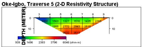
Fig. 7: Inverse resistivity model for Traverse 5 along the landslide axis
