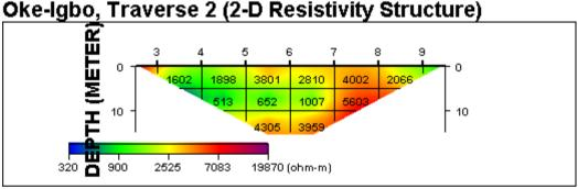
Fig. 4: Inverse resistivity model along Traverse 2 across the landslide
