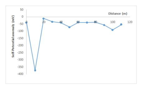
Fig. 12: SP anomaly plot for Traverse 5 along the landslide axis
