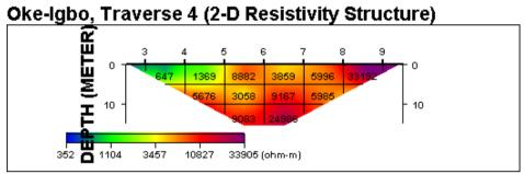
Fig. 6: Inverse resistivity model along Traverse 4 across the landslide
