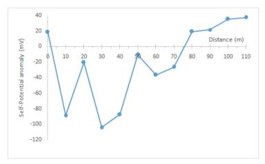
Fig. 8: SP anomaly plot for Traverse 1 across the landslide
