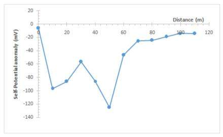
Fig. 11: SP anomaly plot for Traverse 4 across the landslide
