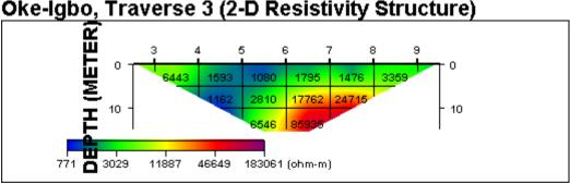
Fig. 5: Inverse resistivity model along Traverse 3 across the landslide
